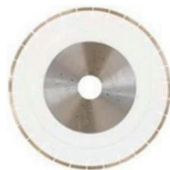
Cutting disc for ULTRA COMPACT MATERIALS with soft bond diamond segments for machines with reduced power (below 20HP). Reinforced body for 45 ° cutting with UCS and LKT materials and glass.
